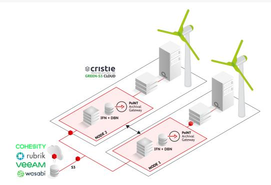
Cristie's GREEN-S3 Cloud provides sustainable and redundant data storage in Germany. WestfalenWIND operates the data centers for the cloud service under the windCORES brand inside its wind turbines in the Paderborn region. They thus use existing infrastructure and are powered directly by renewable energy. A high level of cyber security through location and technology redundancy is central to the GREEN-S3 Cloud.
